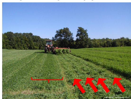
Many wide swath same day haylage efforts are frustrated by mowers that leave small windrows (on right) instead of a uniform wide swath (on left). Twisted knives contribute to the vortex that creates the windrows that inhibit drying.
