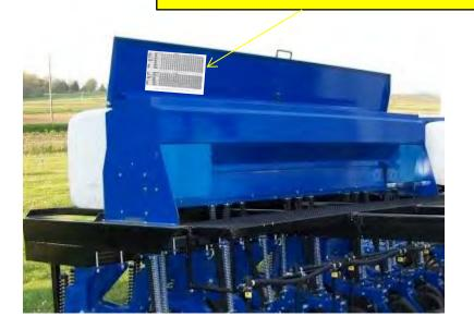
High and low range gears are interchangeable, look for the door sticker to indicate which range
