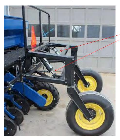
Insert cylinder stops here to assist with leveling if needed
