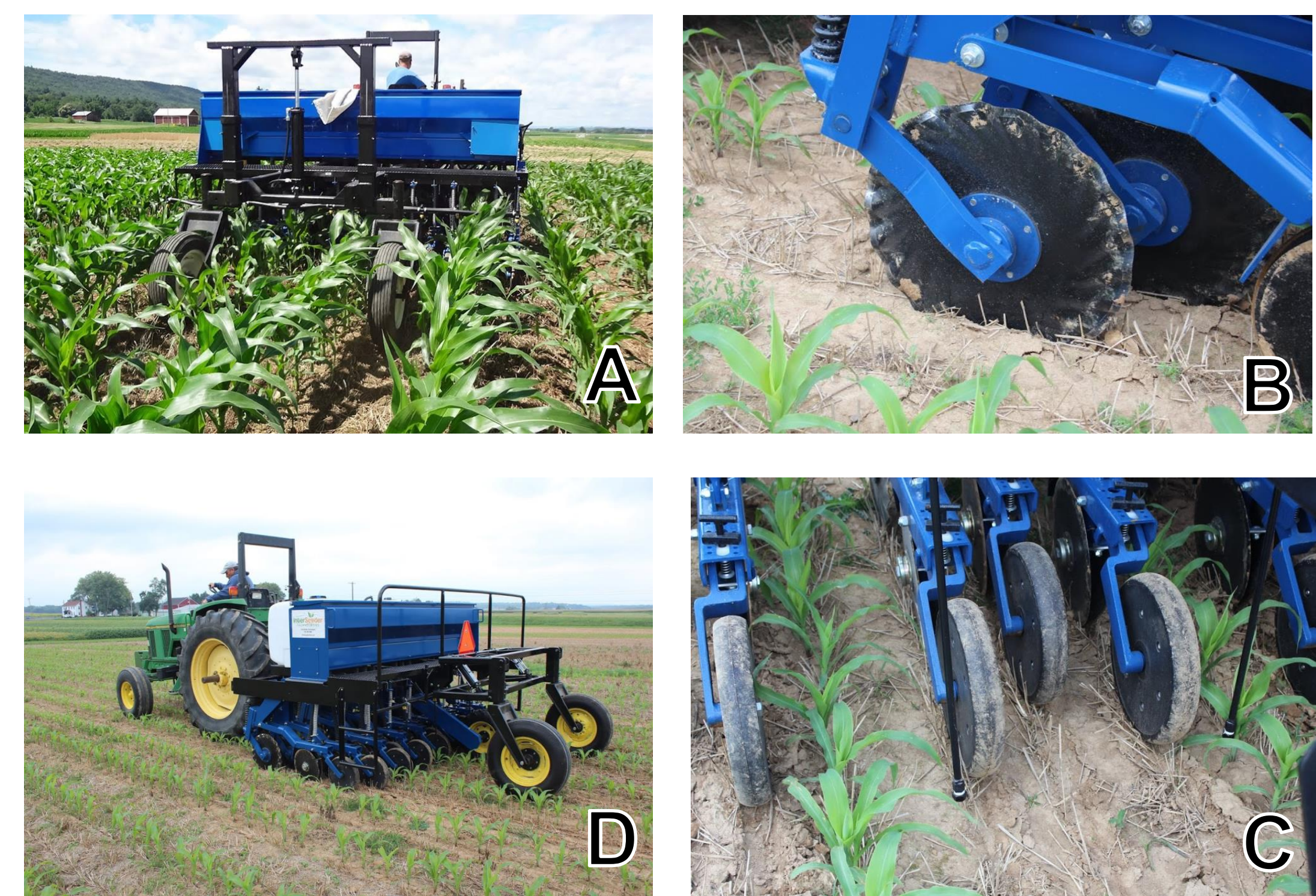
Figure 1. InterSeeder operating components
