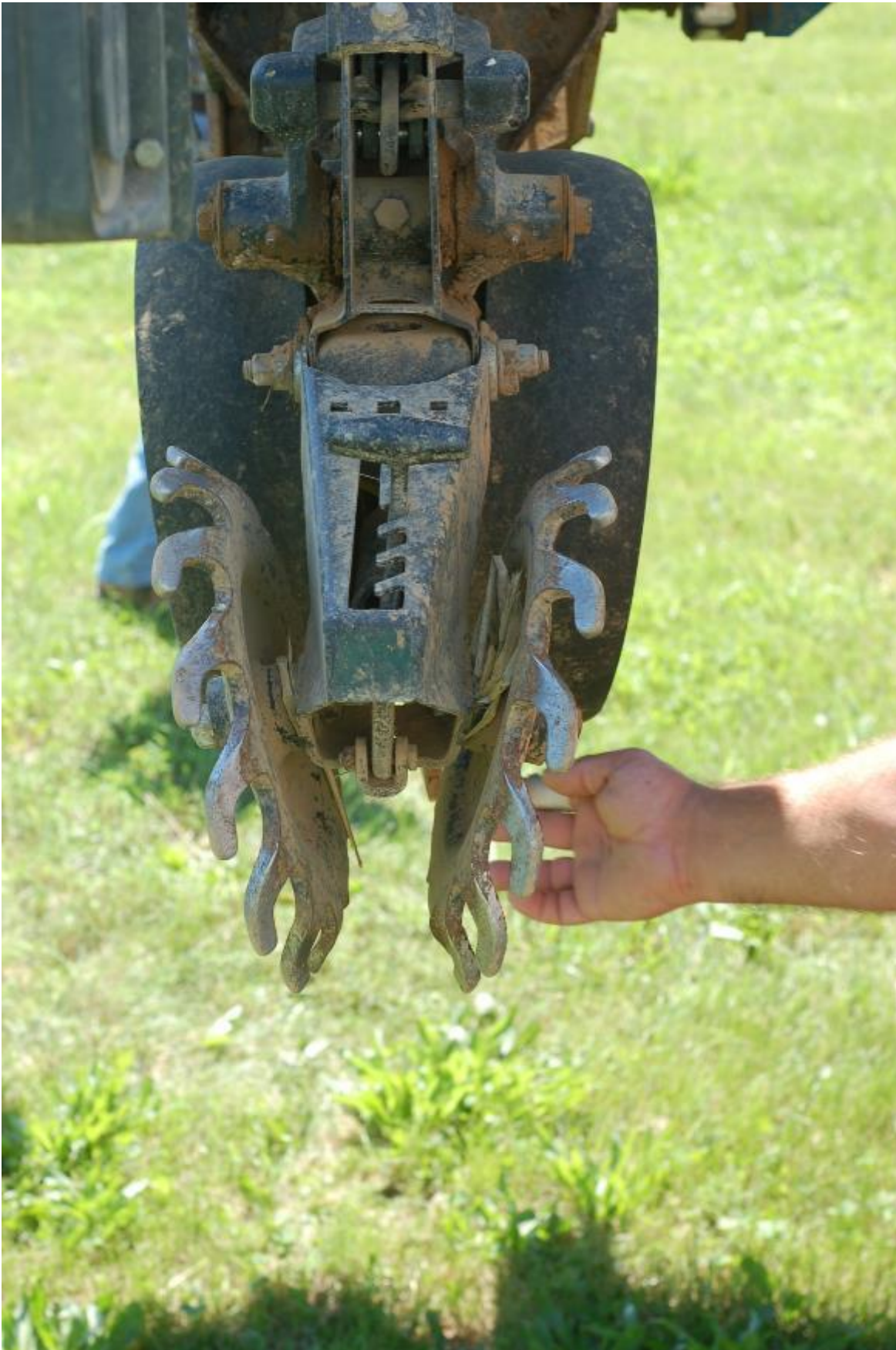
Picture: Close-up of Spider closing wheels.
