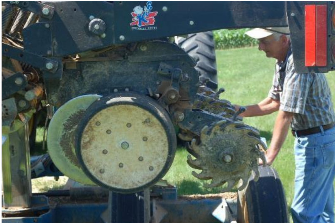
Picture: Jim Biddle shows the dual “spider closing wheels” on his no-till planter.
