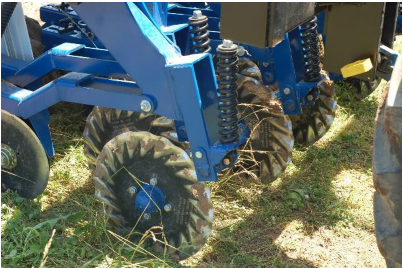
Pictures: Close up of the interseeder No-till Coulters and disk openers for drilling cover crop seeds.
