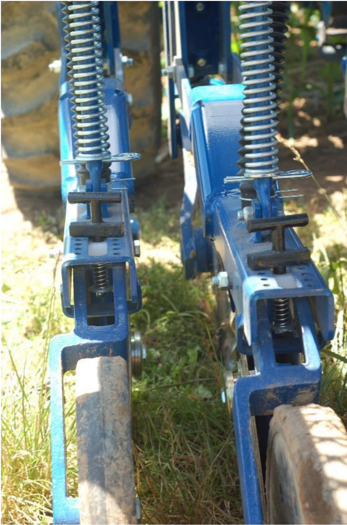
Picture: Close up of press wheels
