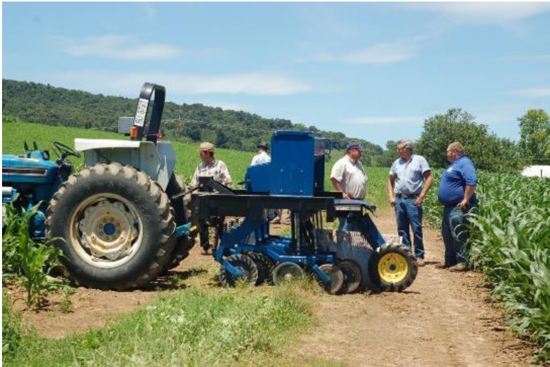
Pictures: Close up of the interseeder No-till Coulters and disk openers for drilling cover crop seeds.
